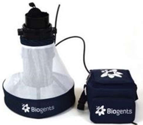
Figure 6. BG-Pro trap in sentinel more, baited with CO 2 (blue bag on the right).
